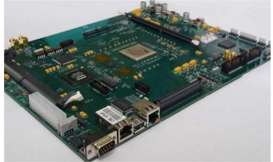
uGMRT correlator and beamformer : a combination of Field Programmable Gate Array (FPGA) and Graphics Processing Unit (GPU).
