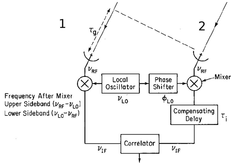
LO provides a single frequency but the RF and IF have a bandwidth; Two sidebands
