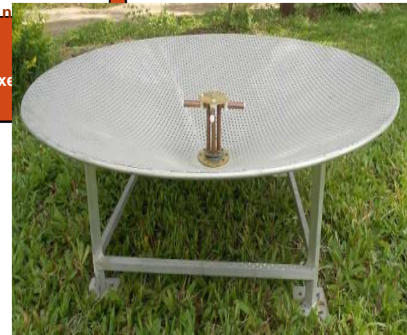
550 - 900 MHz Cone Dipole feed
