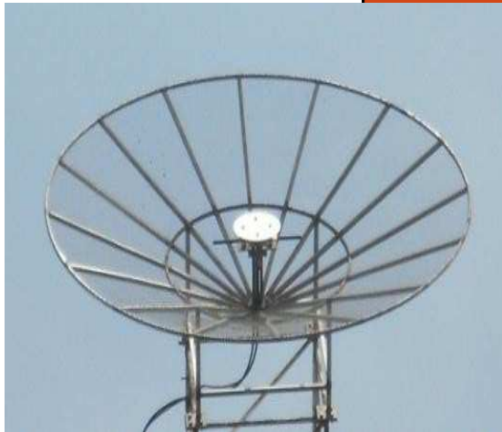
250 - 500 MHz Cone Dipole feed
