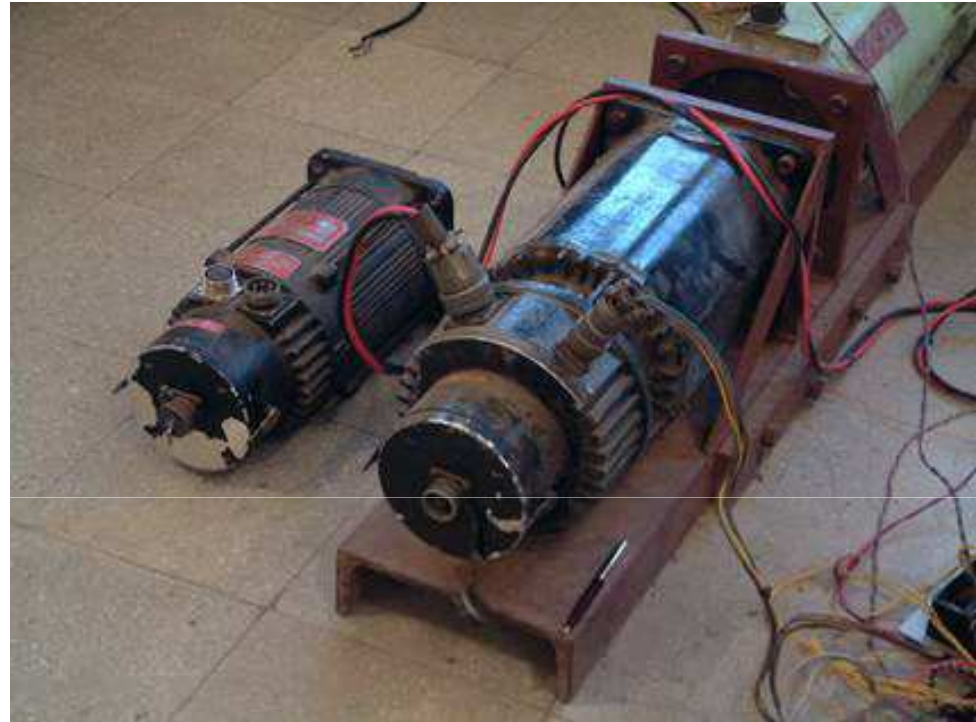
Pair of 6 HP DC servo motors in a counter-torque system for Azimuth and Elevation axes
