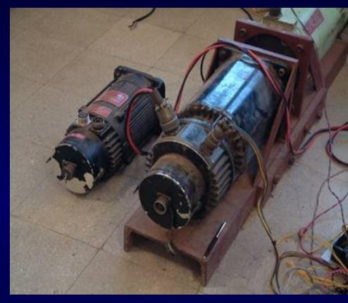
Pair of 6 HP DC servo motors in a counter-torque system for Azimuth and Elevation axes
