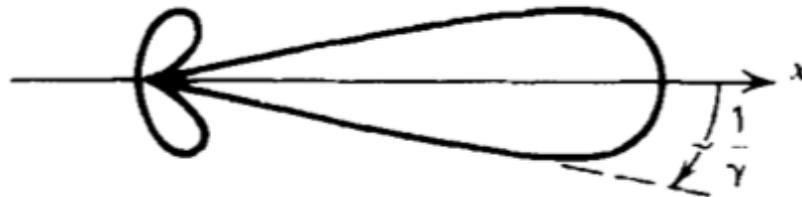
Angular distribution of radiation emitted by a particle with perpendicular acceleration and velocity
