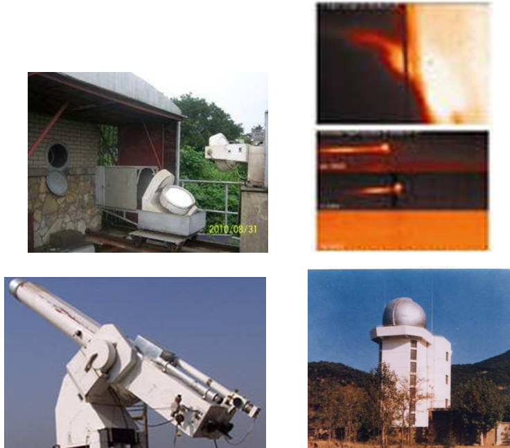
Figure 6. The 2D spectrograph at PMO (upper left) and its 2D spectra at 10830Å(upper right). Ganyu 26cm telescope (lower left) and its dome (lower right).
