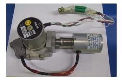
Figure 1. The miniature low power mechanical cooler (RICOR K-508) with space heritage, integrated with a test dewar in TIFR laboratory.
