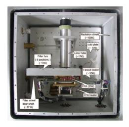
Figure 2. Inside view of the TIRCAM2 dewar system.
