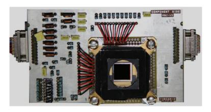
Figure 8. The Fanout Board.
