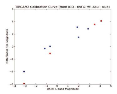
**Figure 14.** Instrumental magnitudes from log of ADUs/sec *versus* actual *L*-band magnitudes from UKIRT, showing linearity of TIRCAM2 in the *nbL*-band (red squares – IGO data, blue squares – Mount Abu data).
