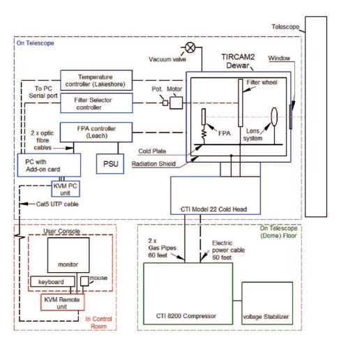
Figure 9. Layout of the TIRCAM2 observational setup.
