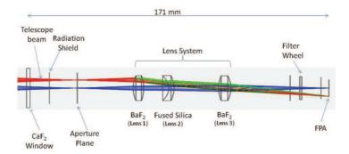
Figure 4. Schematic and Zemax raytrace of TIRCAM2 optics.
