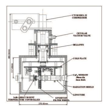
$\textbf{Figure 3.} \ A \ schematic \ of the \ TIRCAM2 \ dewar \ system.$
