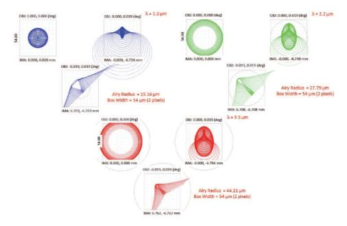
**Figure 5.** Spot diagrams at  $\lambda = 1.2$ , 2.2 and 3.5  $\mu$ m (*clockwise from top left*).
