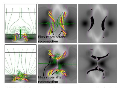
**Figure 4.** MHD simulations of reconnection between two flux ropes. The simulated magnetogram is shown in grayscale with strong positive (negative) flux in white (black). Left panels: 3D view along the flux ropes, showing their cores and ambient field lines. Middle panels: top view. Right panels: top view, showing field line dips in black (adapted from Török et al. (2011)).
