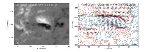
**Figure 1.** (a) MDI LOS magnetogram for AR 10808. White stands for positive polarity and black for negative one; (b) vector magnetogram of the AR from THEMIS observation in MTR mode.
