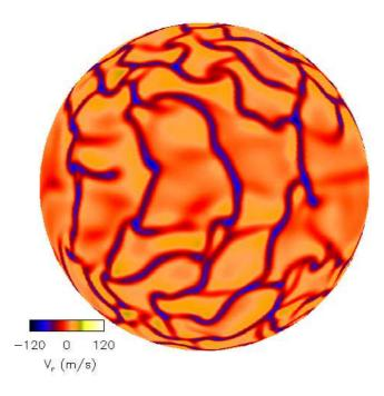
**Figure 3.** From Weber, Fan & Miesch (2011). A snapshot of the radial velocity of the giant-cell convective flow field (used for the thin flux tube simulations) at a depth of 25 Mm below the solar surface.
