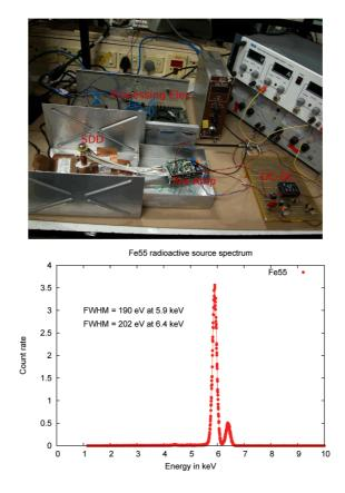
**Figure 2.** Top: Laboratory test setup of the SDD detector. Bottom: Observed Fe55 source spectra showing the Mn K- $\alpha$  and K- $\beta$  spectra clearly separated.
