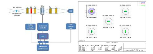
**Figure 2.** Left: Schematic of a dual FP based narrow band imager. Right: Diffraction limited spot diagram of the optical design.
