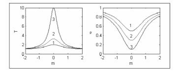
Figure 1. Evolution of a localized initial perturbation (eq. [25]). The temperature and density profiles are shown thrice, corresponding to,  $\beta = 0.9$ , (curve 3),  $\beta = 0.7$  (curve 2),  $\beta = 0.5$  (curve 1).
