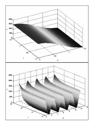
Figure 4. The evolution of temperature for the unstable gas (eq. [58]), the line shows the evolution coming from nonlinear theory,  $T_o = 1500, w = 2$ .
