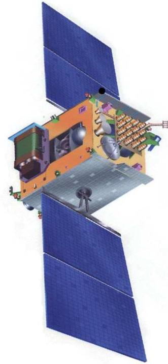
**Figure 1.** A scheme of TAUVEX on board the GSAT-4 spacecraft (S/C), as seen from south-east direction. TAUVEX (the small box) is mounted on the east side of the S/C, and the solar panels emerge from the north and south sides. The panels are rotating on an axis oriented north-south, while the side with the antennas is pointing towards the Earth. TAUVEX MDP can be rotated on its axis oriented east-west. In this chart TAUVEX is pointing to the North.
