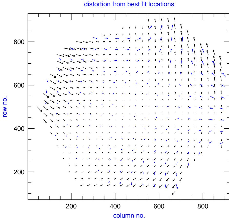
**Figure 5.** Approximation of the TAUVE X distortion during qualification. Detector D13 and 6th order polynomial fit.
