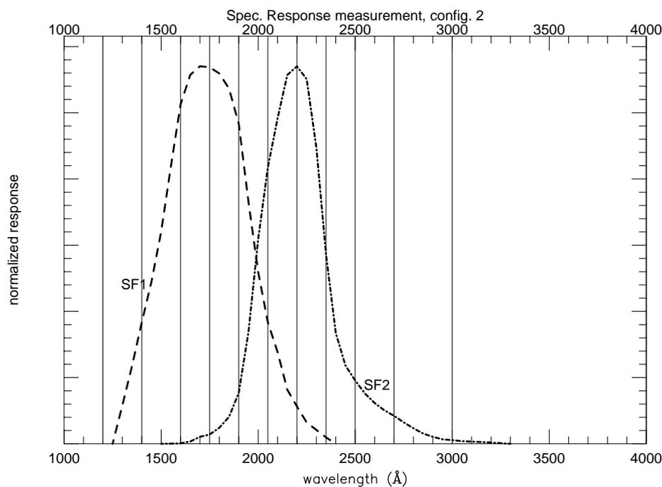
**Figure 8.** Filter profiles and wavelengths to measure for the throughput calibration of SF1 and SF2.
