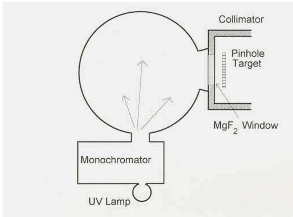
**Figure 3.** Focal plane assembly of collimator with integrating sphere, monochromator, and lamp. The pinhole targets are at the collimator focal plane, in the high vacuum.
