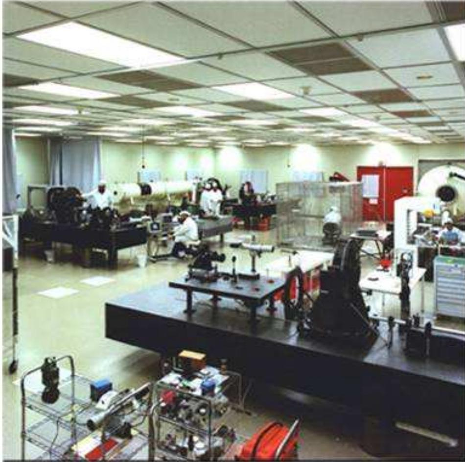
**Figure 1.** Clean room of El-Op. The thermal vacuum chamber is on the right. Its collimator extends out of the clean room into a laboratory. The ambient (clean room) collimator is on the left.
