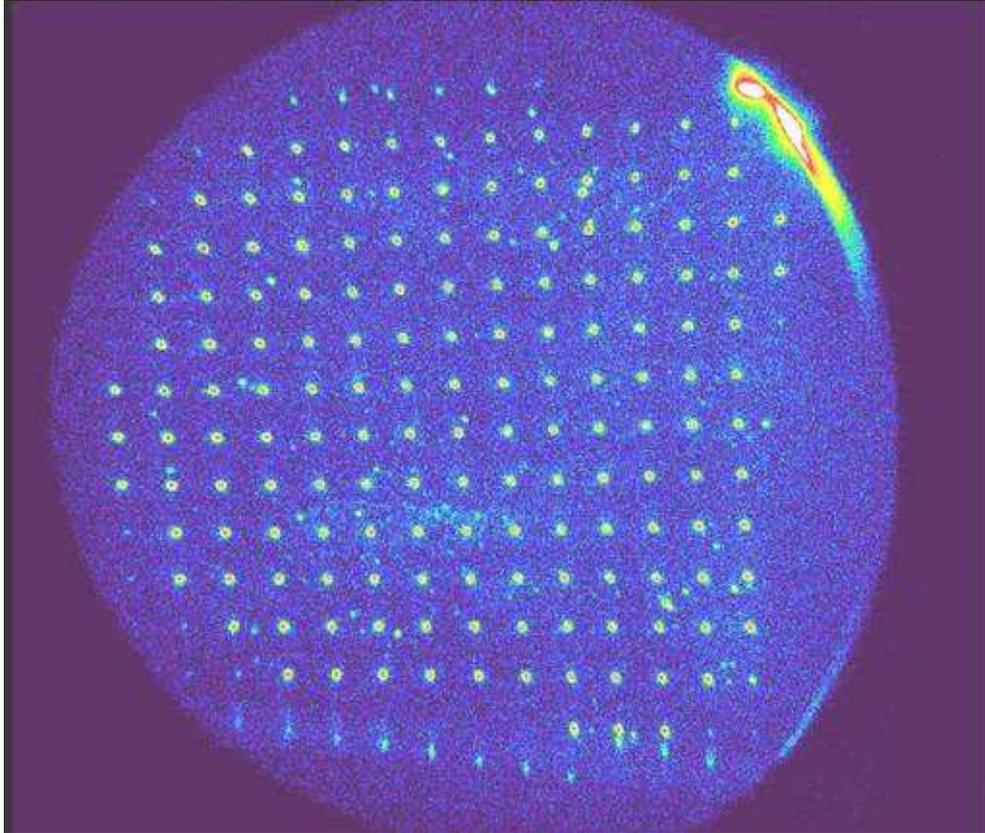
**Figure 4.** Image of distortion matrix obtained during the TAUVE X qualification by combining images from two different TAUVE X orientations.
