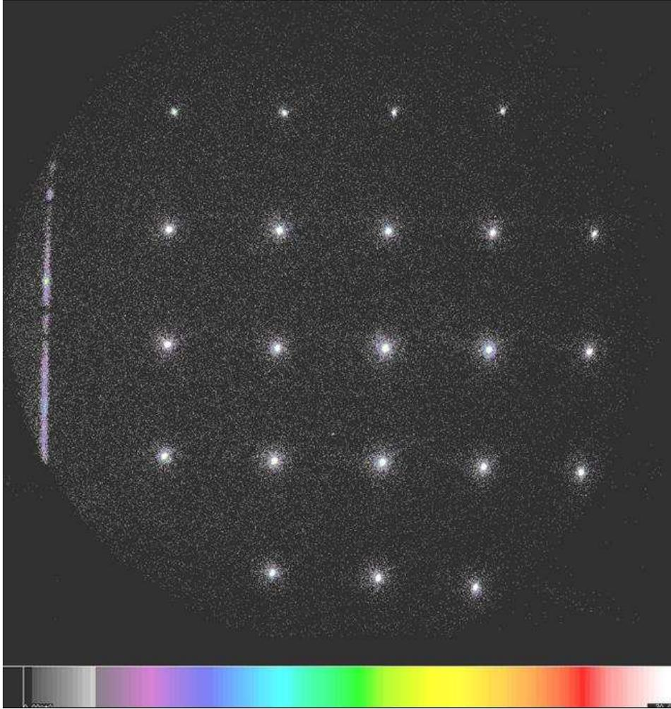
**Figure 6.** Image of the 25 pinhole resolution target obtained during the TAUVEK qualification.
