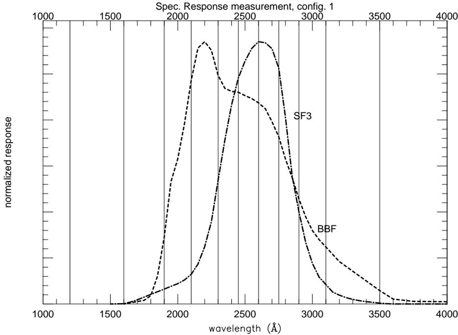
**Figure 7.** Filter profiles and wavelengths to measure for the throughput calibration of BBF and SF3.
