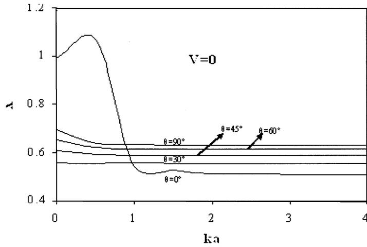
**Figure 2.** The dispersion curve in the absence of flow ( $V = 0$ ).
