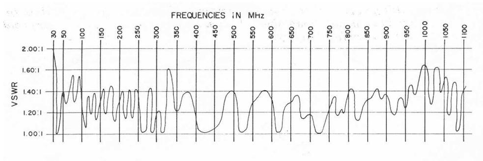
**Figure 2.** VSWR of the LPD antenna in Fig. 1.
