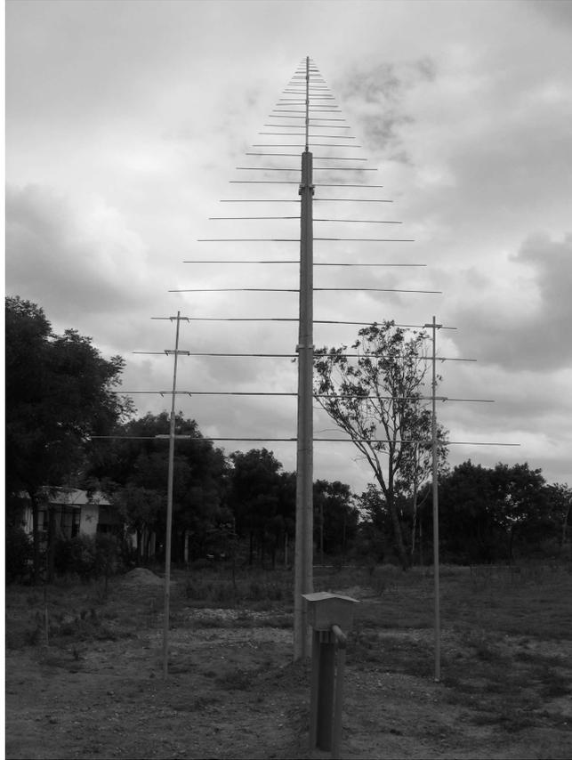
**Figure 1.** The LPD antenna used for the CALLISTO radio spectrometer at Gauribidanur observatory. The box in the foreground houses the amplifier mentioned in the text.
