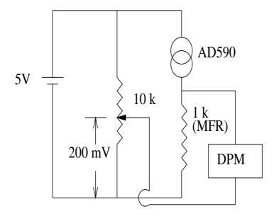
Figure 1. Circuit used for measuring the surface temperature of mirror using AD590 sensor.
