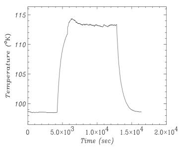
**Figure 4.** Temporal evolution of the surface temperature of the flat of 8 mm thickness, irradiated by solar simulator. The kink near the maximum in the rising part of the curve is due to transient power failure.
