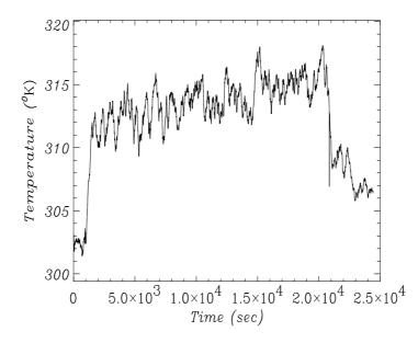
Figure 2. Temporal evolution of the surface temperature of the flat of 8 mm thickness, irradiated by direct sunlight.
