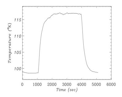
Figure 5. Temporal evolution of the surface temperature of the flat of 2 mm thickness irradiated by solar simulator.
