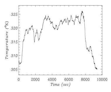
Figure 3. Temporal evolution of the surface temperature of the flat of 2 mm thickness, irradiated by direct sunlight.
