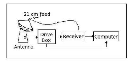
Figure 1: The block diagram of 4 m Telescope system.
