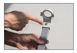
**Step 5:** Loosen the LNB Holder screw and insert the LNB with the Feed side facing towards the dish into it. Tighten the screw so that the LNB stays in place but allow for some slack so that the LNB can be rotated within the holder.
