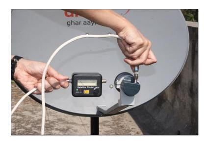
**Step 2:** Take the smaller cable (3 m.) and connect one end to the STB. The cable should be connected to the "IF IN" connector on the back of the STB and NOT to "IF OUT". Connect the other end to the Satellite Finder at the "TO REC" connector marked on the underside of Satellite Finder.
