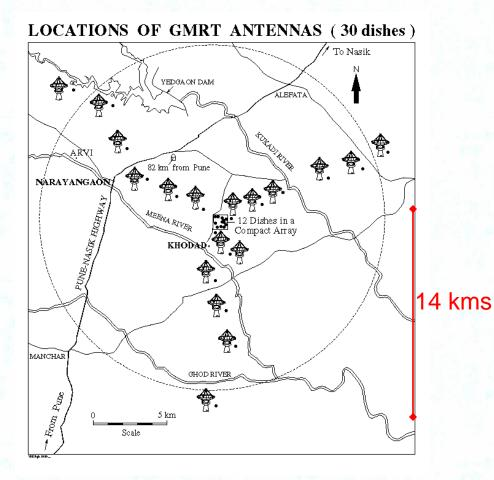
GMRT is located in an array of about 25 km in extent.
