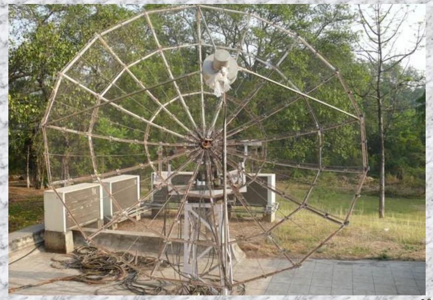
4-m Radio telescope Receiver >Super-heterodyne Receiver
