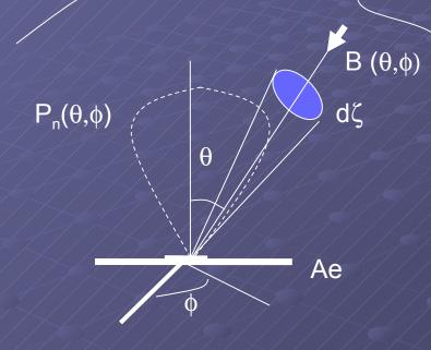
Spectral Power :  $w = Ae B(\theta, \phi) P_n(\theta, \phi) d\zeta$
