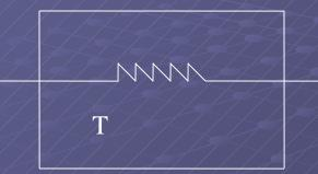
A resistor put in a thermal bath of temperature T will have an output power per unit frequency given by
