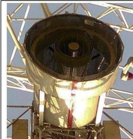
Fig l: 233/610 MHz co-axial feed
