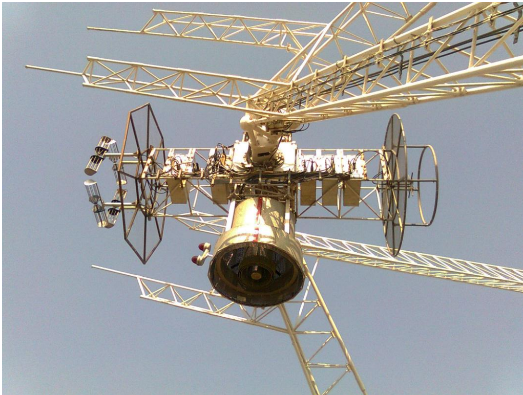
Fig a: Feeds on GMRT turret
