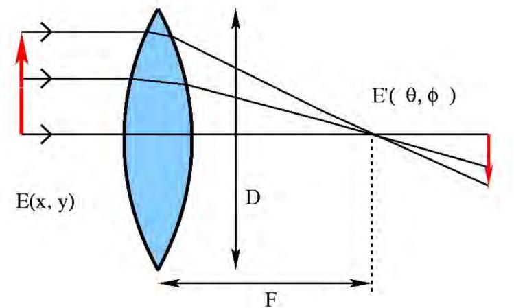
It ensures that the optical path lengths from all points on a plane wavefront (perpendicular to the optical axis) to the focal point are the same.
