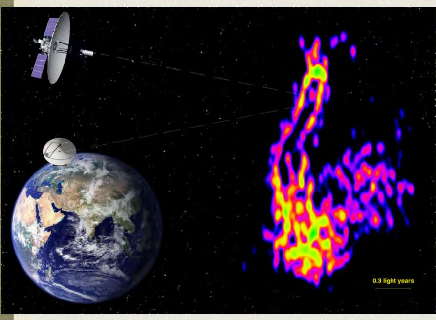
First mission (1997-2003) HALCA 8m dish Best resolution  $\approx 0.1$  mas Freq: 1.6 & 5 GHz New mission (2011) RadioAstron - 10m dish Max. Baseline = 350,000 km Freq: 0.325, 1.6, 5, 22 GHz Perseus A with ~50
