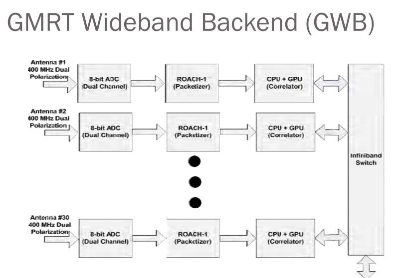
Real-time (800 MHz, 30 antenna, dual polarization) Correlation and Beamforming is split across several signal processing platforms (FPGA and GPU)
