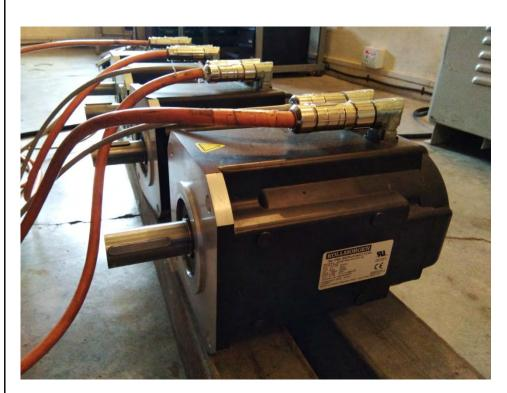
Brushless DC motors – Azimuth and Elevation
