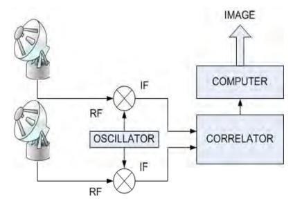
**Basic two-element Interferometer**
