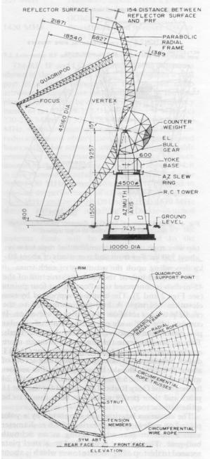
Alt-Azimuth mount with ~3.5m dia azimuth bearing !
