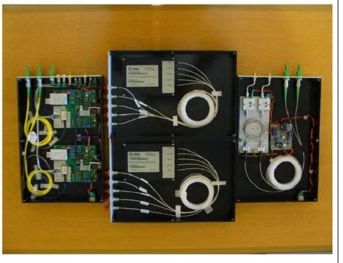
LASER Transmitter, Optical Multiplexer, Optical receiverIAS Summer SchoolDWDM based system3/7/2018Image Courtesy: OFC Group
