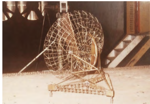
Wind tunnel testing of GMRT antenna at IISC aerospace engineering department.
