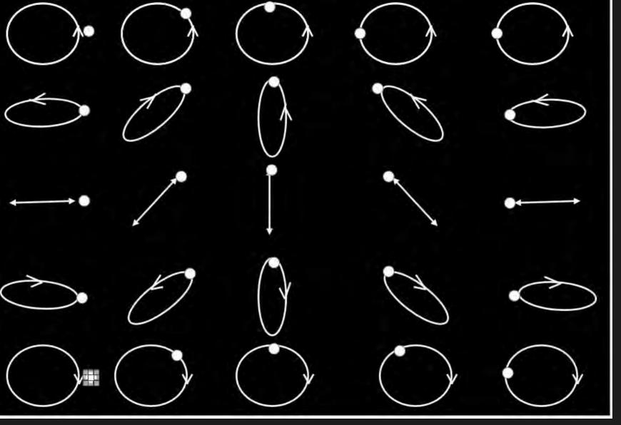
We need a phase convention to define Stokes visibility between differently polarised antennas
