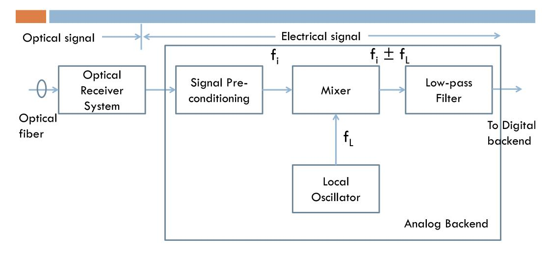
Analog backend amplifies the signal, converts from radio frequency to baseband through frequency heterodyning and provides desired bandwidth signal to the digital system
