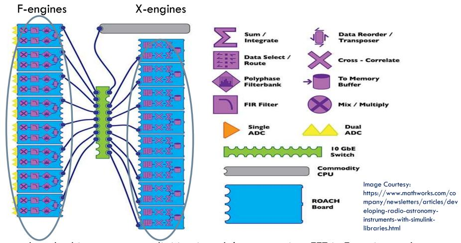
Commonly used method is to carry out digitization, delay correction, FFT in F-engine and multiplication and accumulation in X-engine. High speed data connectivity is required between the F & X engines
