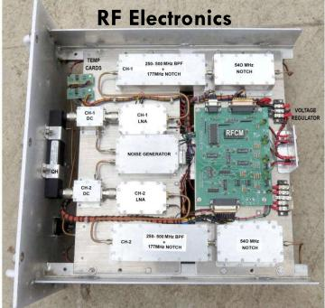
Multi-stage amplification (~60 dB) at prime-focus
