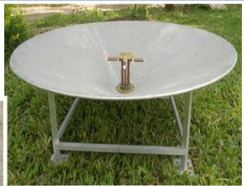
550-900 MHz Cone Dipole feed
