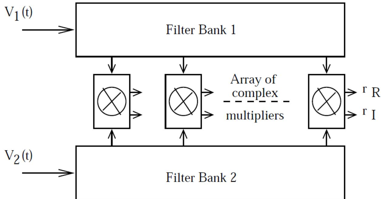
The band limited signal is decomposed into spectral components using a filter bank and each filter output is cross correlated with the corresponding one from the other using a complex multiplier.
