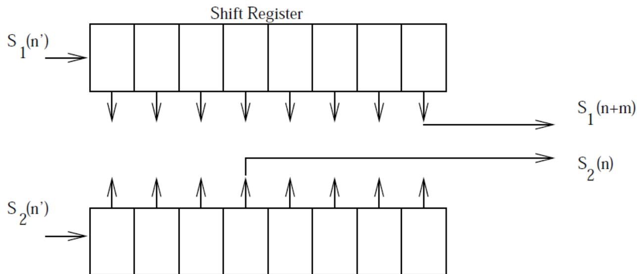
Delay implementation using shift registers
