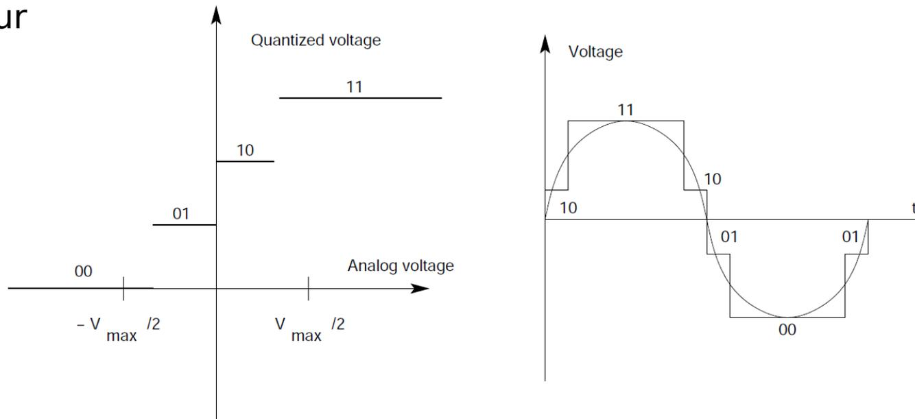
Quantization distorts the sampled signal affecting both the amplitude and spectrum of the signal.
