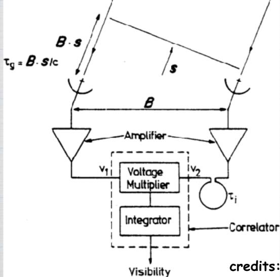
The interference pattern is directly related to the source brightness: (for small fields-ofview) the complex visibility is the 2D Fourier transform of the brightness on the sky.
