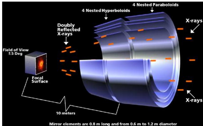
**Figure 2.** Schematic representation of the Giacconi-Rossi concept as applied to the Chandra X-ray Observatory mirrors. In Chandra the focal surface contains the High Resolution Camera and the Advanced CCD Imaging Spectrometer on a translation table (<http://chandra.harvard.edu/graphics/resources/illustrations/excmirrors-72.jpg>).
