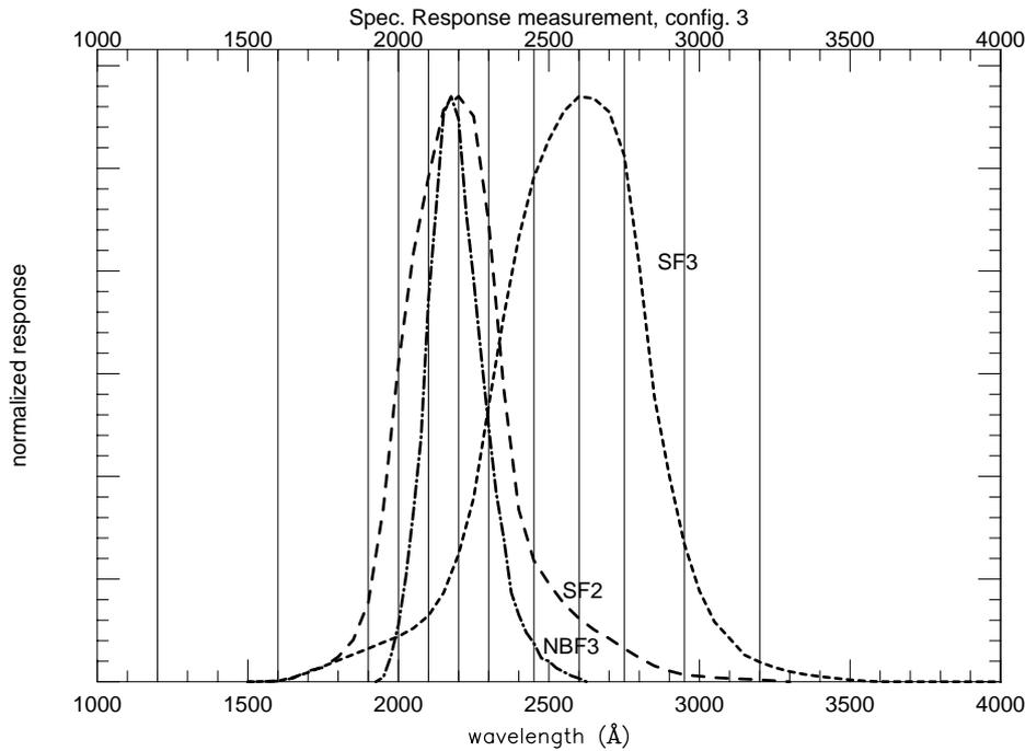
**Figure 9.** Filter profiles and wavelengths to measure for the throughput calibration of NBF3, SF2 and SF3.
