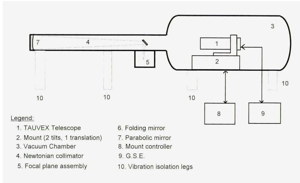
**Figure 2.** Schematic diagram of the thermal vacuum chamber with collimator for TAUVE X calibration.
