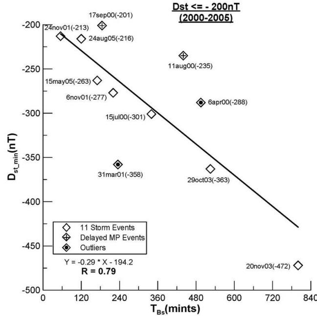
**Figure 2.** Above figure represents the dependence of storm intensity on  $T_{Bs}$ , defined as the duration of post-shock southward  $B_z$  during the storm period of events.
