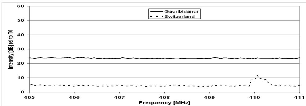
**Figure 7.** Same as Figs 3-6 but in the frequency range 405-411 MHz. The band 406.1-410.0 MHz is shared by radio astronomers with other authorized users.
