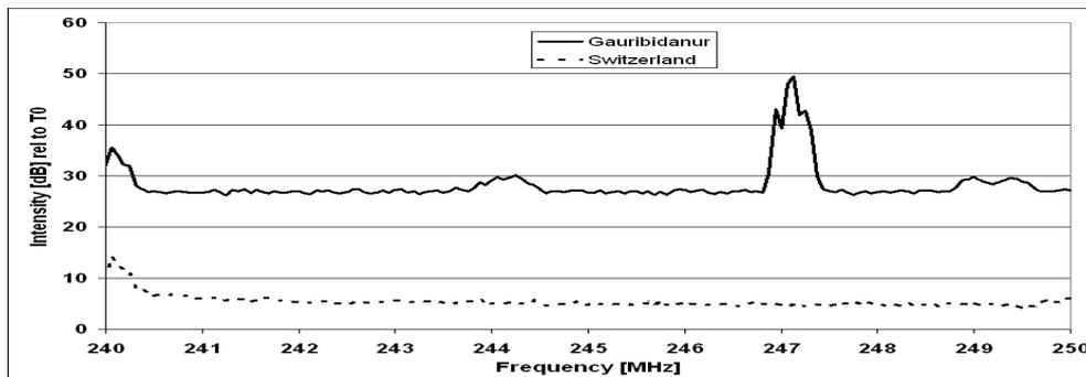
**Figure 5.** Same as Figs 3 & 4, but over the band 240-250 MHz. The large hump near 247 MHz in the Gauribidanur spectra is due to GRH local oscillator signal.
