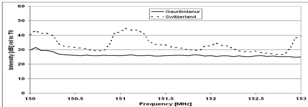
**Figure 4.** Same as Fig. 3, but over the band 150-153 MHz. Frequencies from 150.05 till 153.00 MHz are primarily allotted for radio astronomy observations.
