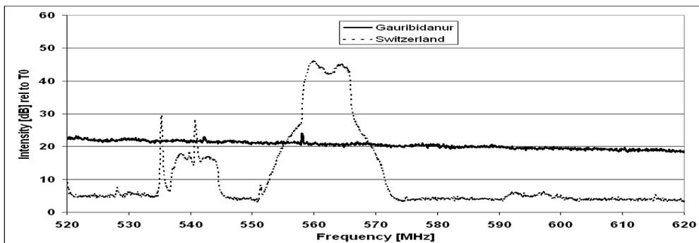
**Figure 8.** Same as Figs 3-7, but over the band 520-620 MHz. The broad regions of interference in the Switzerland spectra are due to digital TV transmission. The range 608-614 MHz is shared with broadcast services as mentioned above.
