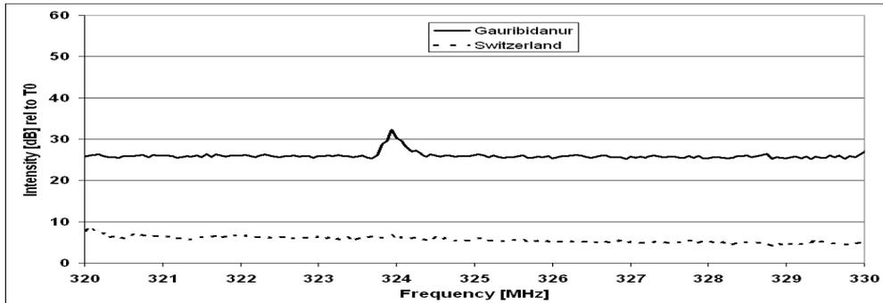
**Figure 6.** Same as Figs 3-5 but over the band 320-330 MHz. The spectral range 322.0-328.6 MHz is a primary radio astronomy band for Deuterium spectral line observations. The hump near 324 MHz is due to local interference at the Gauribidanur observatory.
