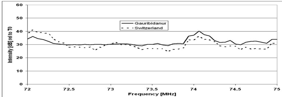
**Figure 3.** A comparison of the RFI situation in Gauribidanur and Switzerland in the frequency range 72-75 MHz. The band 73.0-74.6 MHz is shared by radio astronomers and fixed/mobile radio-communication users.
