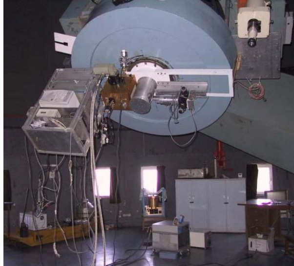
Figure 1. TIRCAM at the Cassegrain focus of the Mt. Abu Infrared Telescope. The dewar, the drive electronics (on the adjoining rack) as well as the closed cycle cryocooler (cold head on the dewar, Helium gas pipe lines & the compressor on the ground) are visible.
