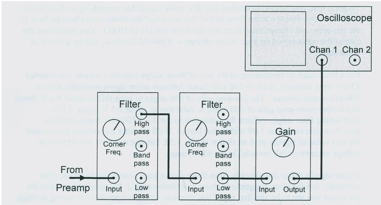
Figure 1: Connection Diagram
