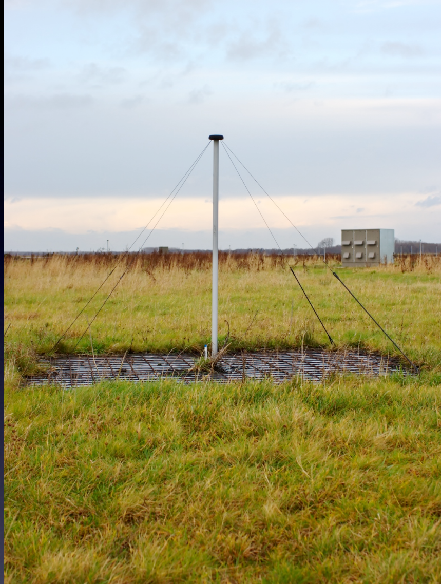
A LBA dipole (10-90 MHz), part of the sparse aperture array
