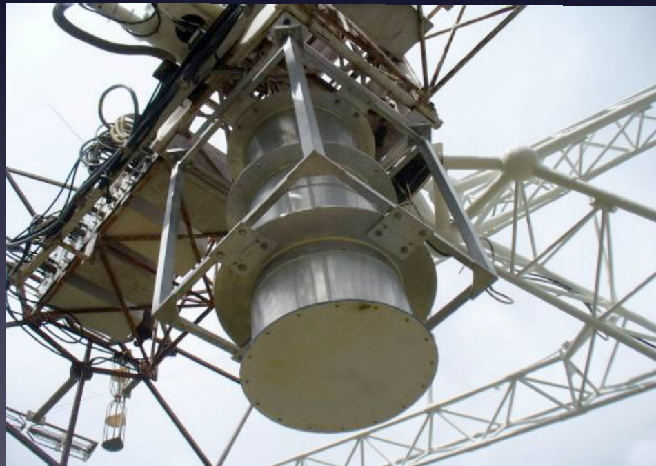
New 550-900 MHz feed for the upgraded GMRT
