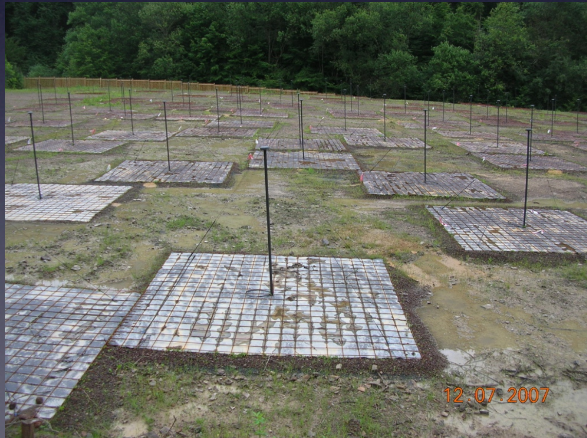
A LBA dipole (10-90 MHz), part of the sparse aperture array
