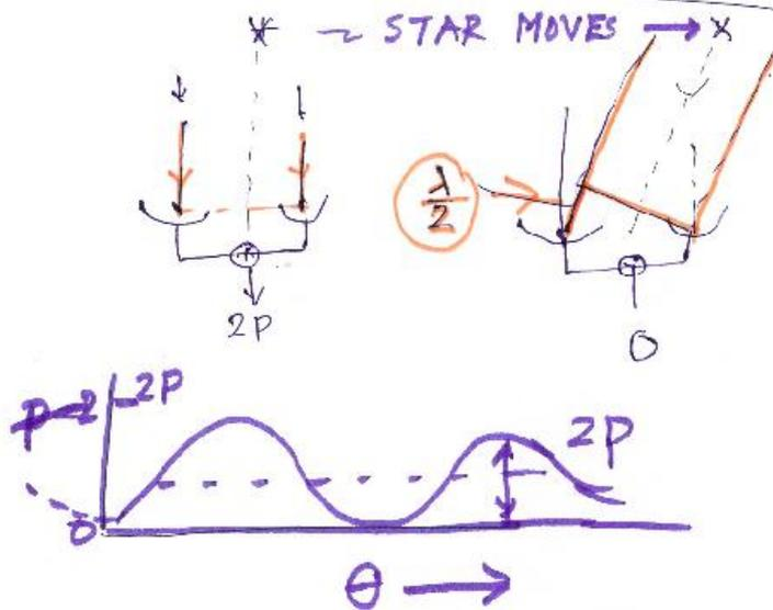
A basic radio interferometer consist of pair of antennas that measure one Fourier component of the radio or optical source.
