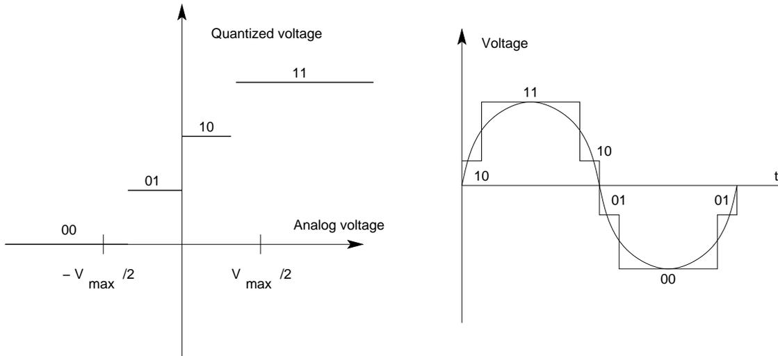
Figure 8.1: Transfer function of a two bit four level quantizer. The *binary* numbers corresponding to the quantized voltage range from 00 to 11. Quantization of a sine wave with such a quantizer is also shown.
