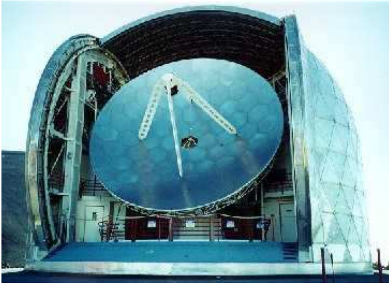
Figure 3.3: The Caltech Sub-millimeter Observatory (CSO) at Mauna Kea in Hawaii. The telescope operates in the the sub-mm wavelength range.
