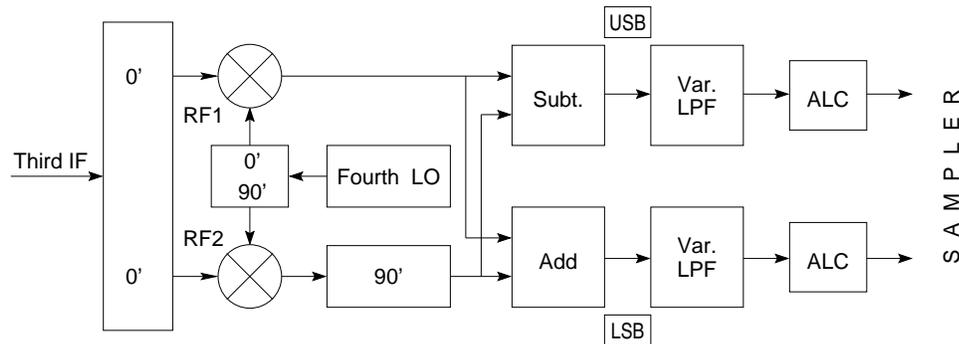
Figure 23.4: A simplified block diagram of the base-band processing at the GMRT.
