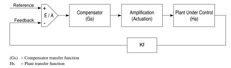
Figure 20.1: Closed loop control system.
