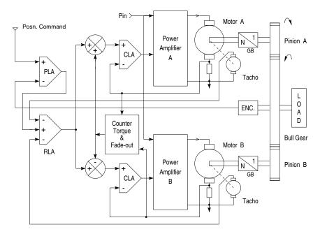
Figure 20.5: Dual drive position control system.
