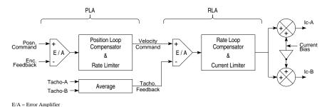
Figure 20.3: Rate loop amplifier.
