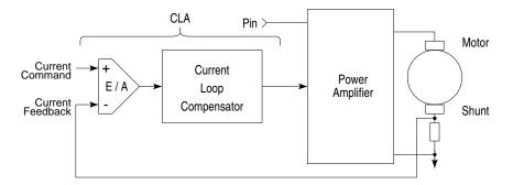
Figure 20.4: Current loop amplifier.
