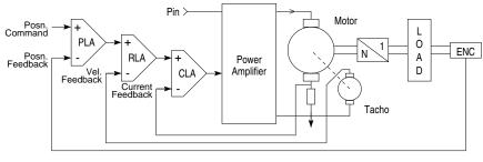
GB = Gear box. ENC = Encoder. PLA = Position Loop Amplifier. RLA = Rate Loop Amplifier.
