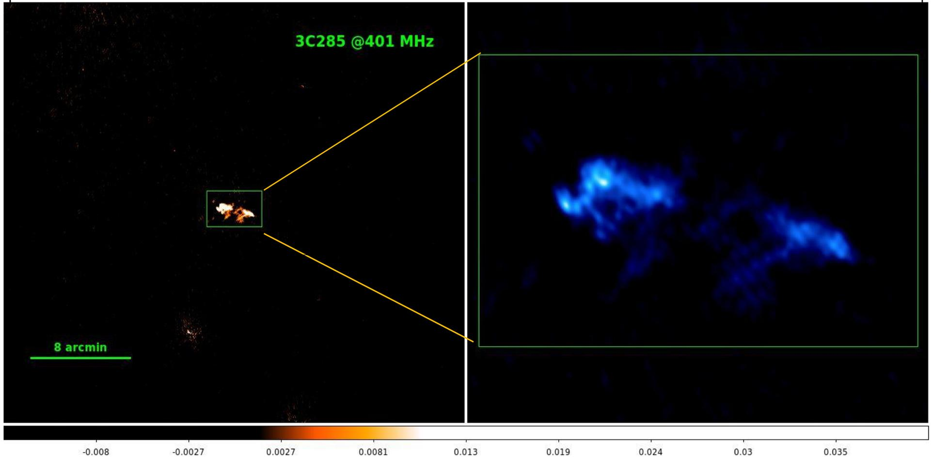
**3C285 observed for about 3 hours using 11 broadband antennas, 300 MHz RF, 200 MHz bandwidth, 2048 spectral channels. RMS noise: 0.6 mJy,  $\sim 5.4$  arcsec resolution**
