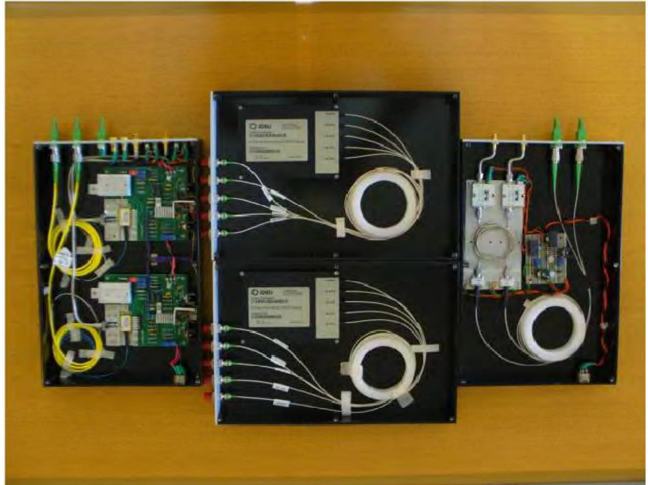
**LASER Transmitter, Optical Multiplexer, Optical receiver**
