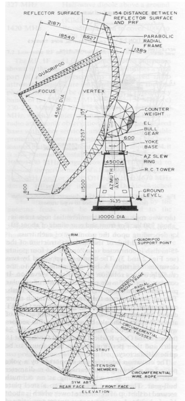
Alt-Azimuth mount with ~3.5m dia azimuth bearing!
