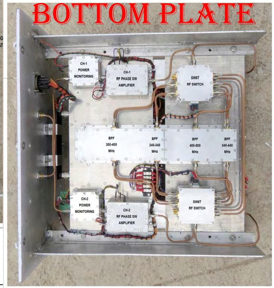
Front-end box installed at the prime-focus consists of polarizers, low-noise amplifiers, filters and monitoring and control circuitry
