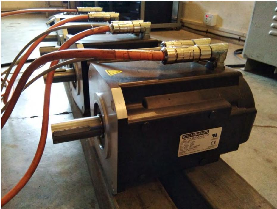
Brushless DC motors – Azimuth and Elevation
