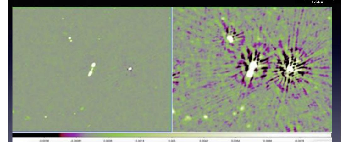
240 subband (48MHz BW) facet calibrated resolution ~ 5" rms noise: 85 uJy/beam 300 subband (70MHz BW) not facet calibrated resolution ~ 18" rms noise: 160 uJy/beam
