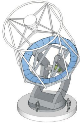
**Figure 1.** The sketch of the CGST which is designed as the ‘ring solar telescope’.
